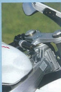
Steering damper to keep the Mito in line.
